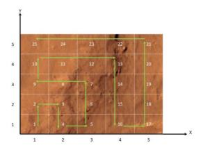
Given this navigation strategy it is easy to predict the time spent to arrive at the target position (x,y). When rover is at (2,3), the rover took 8 seconds. And when it was at (5,4), the rover was at the 20th second of the movement.
